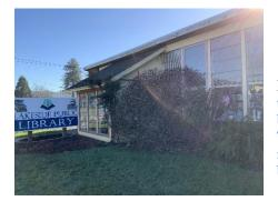
**Note:** Observed the vegetation around the building is within 1 foot from the exterior walls. It is recommended that the landscaping be trimmed back to provide 2 feet of clear space.
